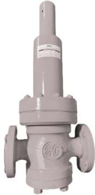
Direct Acting Downstream Pressure Regulating Valves – also, called as Pressure Reducing Valves – are meant for reducing the source pressure and regulating the outlet / downstream pressure at the pre-determined set value required for the processes. With direct acting Regulators precise pressure control can be achieved at specified process requirements.
